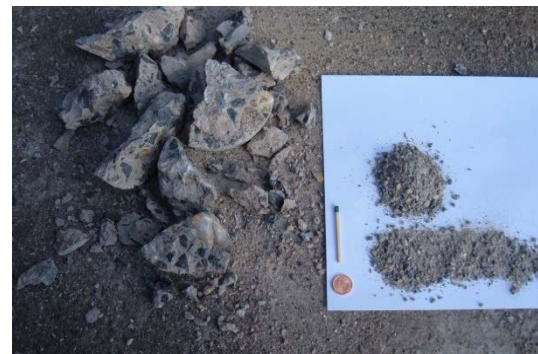
Fig. 2: Pre-crushed drilling core
