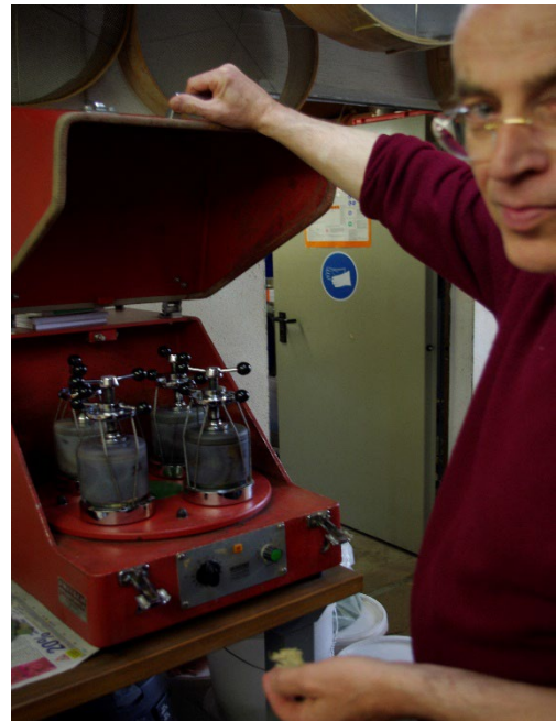
Fig. 3: Dr. Kremer using the Planetary-Ball Mill PULVERISETTE 5
