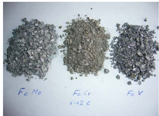
Fig. 2: Sample after comminution with the Jaw Crusher PULVERISETTE 1
