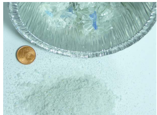
Fig. 1: PET bottles comminuted with 1 mm sieve at 16.000 rpm
