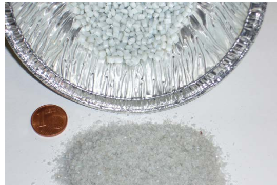
Fig. 2: Granulate comminuted with 1 mm sieve at 10.000 rpm
